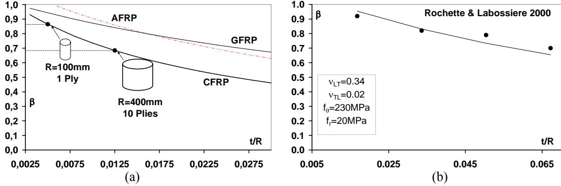
Figure 1. (a) Predicted efficiency factors for columns strengthened with AFRP, GFRP and CFRP- (b) Predicted efficiency factor vs. experimental outcome: Rochette & Labossiere (2000)
