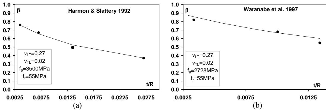
Figure 2. Predicted efficiency factor vs. experimental outcome: (a) Harmon & Slattery (1992) – (b) Watanabe et al. (1997)
